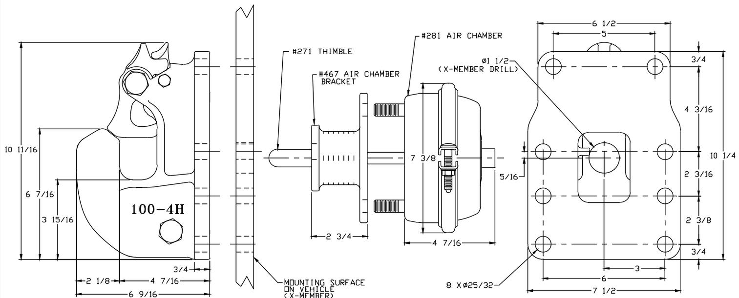
Pushrod length is 3 1/8 in. (79 mm) plus thickness of mounting structure for standard installations as illustrated.
