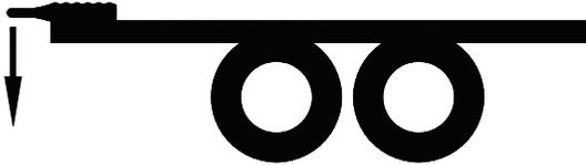
"Tongue Weight Capacity" is the maximum expected weight at the drawbar eye. If a hinged drawbar is used, the maximum weight will be approximately 1/2 the overall drawbar weight. If a non-hinged drawbar is used and the actual tongue weight is not known, you can approximate the weight by multiplying the GVWR of the towed trailer by 15%. However, each application is unique and the best practice is to weigh the tongue when the trailer is loaded to its GVWR.
