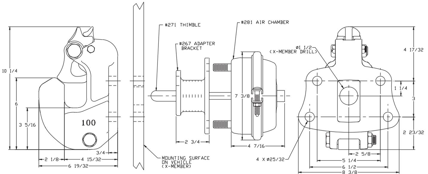
Pushrod length is 2 7/8 in. (73 mm) plus thickness of mounting structure for standard installations as illustrated.
