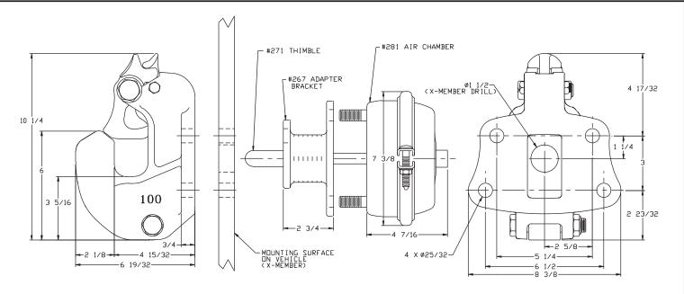
Pushrod length is 2 7/8 in. (73 mm) plus thickness of mounting structure for standard installations as illustrated.
