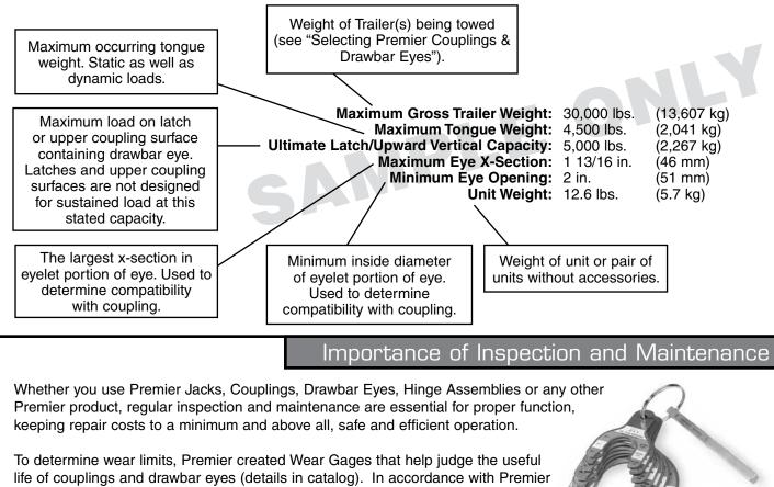
life of couplings and drawbar eyes (details in catalog). In accordance with Premier and the Federal Motor Carrier Safety Regulations, these were designed to identify wear at the critical percentages of 18% and 20%, by measuring the crosssection of coupling hooks (horn) and drawbar eye loops. 18% wear indicates that
