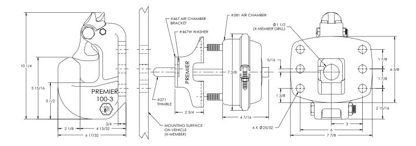
Pushrod length is 3 1/8 in. (79 mm) plus thickness of mounting structure for standard installations as illustrated.
