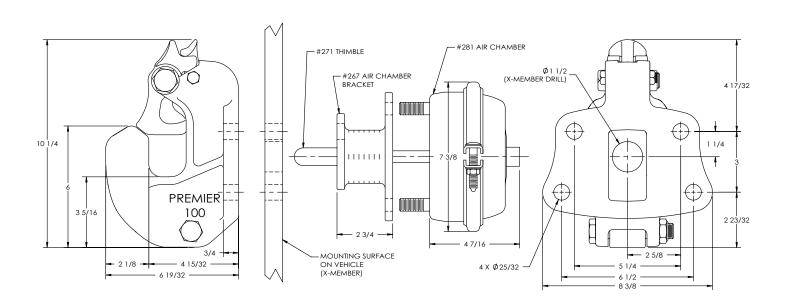
Pushrod length is 2 7/8 in. (73 mm) plus thickness of mounting structure for standard installations as illustrated.
