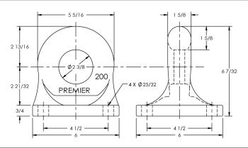
**Inside Diameter:** 2 3/8 in. (60 mm) **Unit Weight:** 16 lbs. (7.3 kg)
