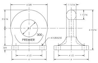
**Inside Diameter:** 3 in. (76 mm) **Unit Weight:** 19.5 lbs. (8.9 kg)
