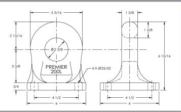
**Inside Diameter:** 2 3/8 in. (60 mm) **Unit Weight:** 19.1 lbs. (8.7 kg)
