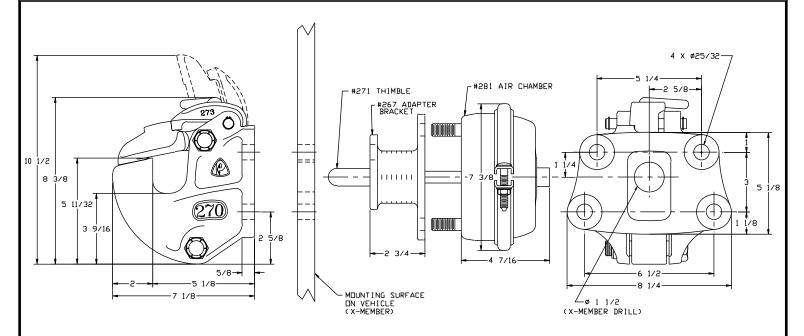
Pushrod length is 3 5/8 in. (92 mm) plus thickness of mounting structure for standard installations as illustrated.
