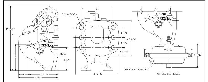
Pushrod length is 2 3/8 in. (60 mm). Not for use with rear mount air can.
