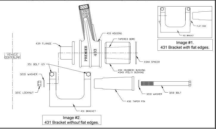
This document is to assist in the replacement of the 430/430A Hinge Assembly components that had previously been installed. <u>Because the 430/430A Hinge Assemblies operate in pairs, the service instructions below are to be followed simultaneously, for each hinge.</u>
