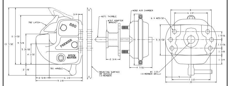
Pushrod length is 5 3/8 in. (137 mm) plus thickness of mounting structure for standard installations as illustrated.
