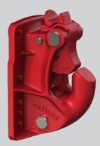
A **pintle hitch** is basically a pincer-type device that closes around a lunette ring or drawbar eye mounted on a trailer. Its larger weight capacity (up to 150,000 pounds GTW) is a tremendous edge, useful for even the most demanding loads. The large lunette ring/drawbar eye makes it ultra-easy to connect, giving a lone driver a more forgiving option.
